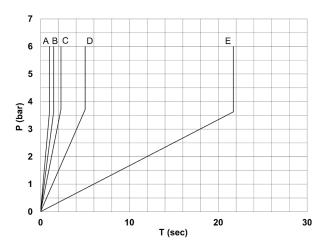
Pressurisation times as to the n° of turns of the regulation screw, with downstream volume of 5 litres. A = 5 turns; B = 4 turns; C = 3 turns; D = 2 turns; E = 1 turn. "K" =  $n^{\circ}$  of turns of the regulation screw required to obtain the required pressurisation time with an inlet pressure of 6 bar. Variations of the inlet pressure can cause deviations of the pressure time by ± 20%. K = t/V where: V = volume of the downstream system in litres; t = desired pressuring time in seconds.
