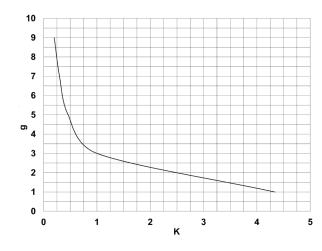
Example: MC104-AV V = 5 litres t = 16 seconds K = 16/5 = 3.2g = number of turns Using in the graph this value K, the number of turns of the regulation screw will be Example: MC238-AV - MC202-AV V = 5 litres t = 16 seconds K=16/5=3,2g = number of turns Using in the graph this value K, the number of turns of the regulation screw will be
